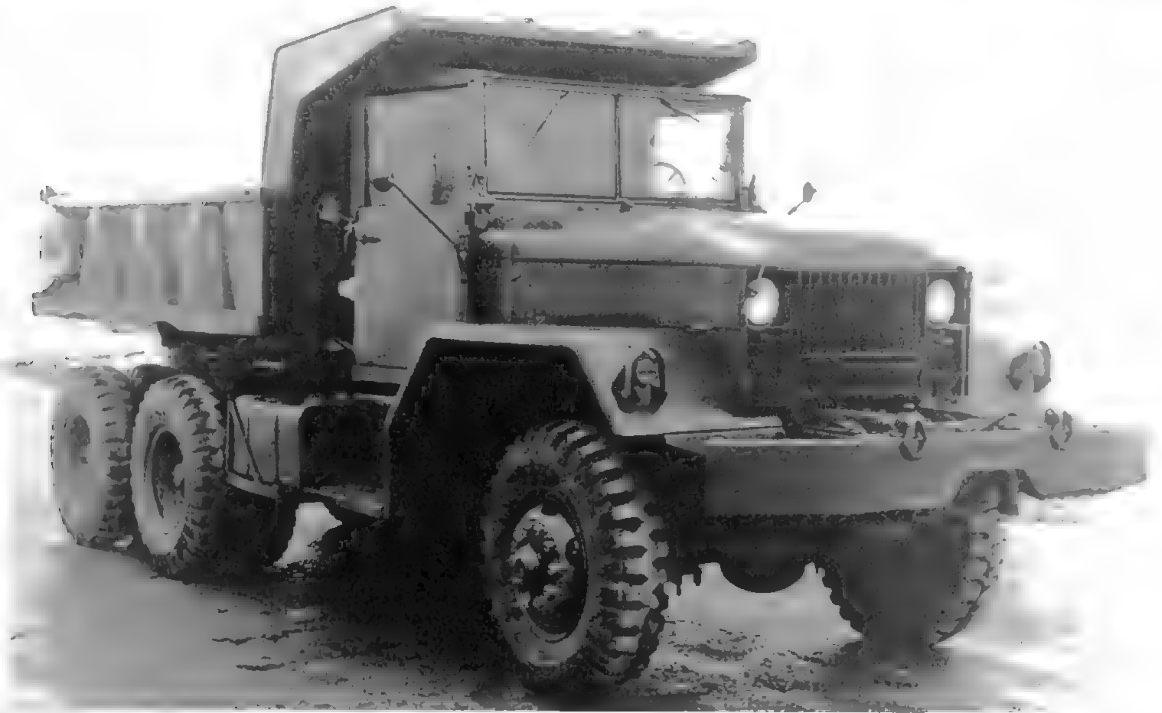
The M51 dump truck was designed to transport 5 cubic yards of material. Two hydraulic cylinders lifted the bed. (Photo courtesy of the Patton Museum)
